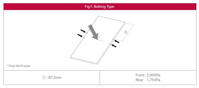
Note) When installed Fig.7, follow the NEXTracker's recommended applied torque and materials to fasten the modules.
