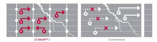
Cello Technology increases long-term performance. Even if micro-cracks naturally occur, Cello Technology will mitigate the degradation of performance with more electrical paths.
